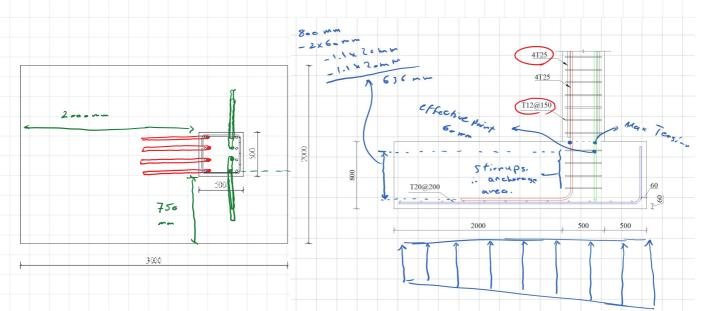
$$c 35/45 \rightarrow 73.1 \rightarrow f_{efk,0.05} = 2.2 \text{ Mpa} \rightarrow f_{e+d} = \alpha_{e+} \cdot \frac{f_{e+k,0.05}}{8c} = 1.47 \text{ Mpa}$$
