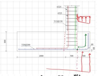
$$L_{b,rq} = \frac{4}{4} \cdot \frac{f_{1d}}{f_{6d}} = \frac{20}{4} \times \frac{435}{3.3} \approx 660 \text{ mm}$$
