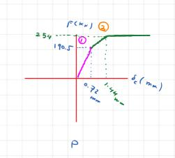
P=160 KN / 190. 5 KN -> Two rods are loaded less than their yielding load.
