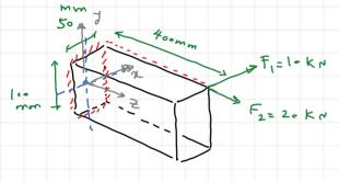
$$F_{1}: \begin{cases} F_{K} = 10KN \\ M_{g} = 10KN \times 0.4m = 4KN.m \\ T = 10KN \times 0.05m = 0.5KN.m \end{cases}$$
